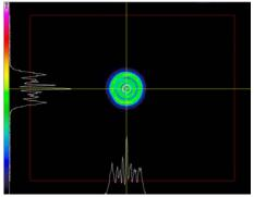
*Comments:* The Aligner is aligned. Diffraction pattern is symmetric. The center of rings coincides with the crosshair.
