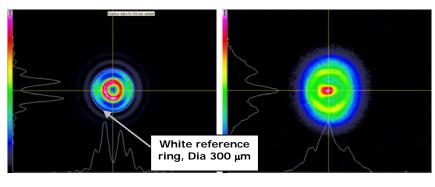
*Important*: It is convenient to use a reference ring like white ring of 300 µm diameter on the above and below pictures.
