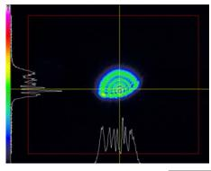
*Action*: to do tilt in vertical direction with checking the spot with camera to provide symmetric diffraction pattern being centred with the crosshair.
